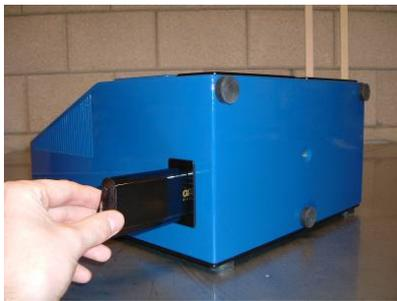
1. Only the batteries and power supply provided can be used with the Proliner. Make sure that the batteries are inserted with the connector pins on the right side, otherwise you could damage the Proliner. The batteries will last up to 2 hours. When the machine is started, the indicator shows what battery life is left. When the capacity reaches 10%, a repetitive beep will be heard until the Proliner shuts down. When the Proliner is connected to a power socket, it will charge the inserted battery.
