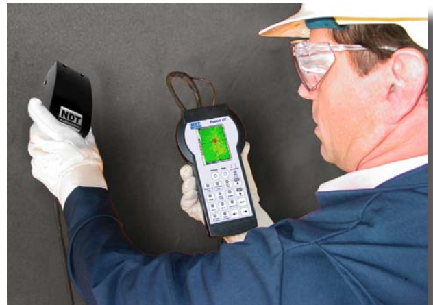
Dual-axis, dry-coupled scanner connects directly into the hand-held Pocket UT System for full C-Scan data acquisition.
