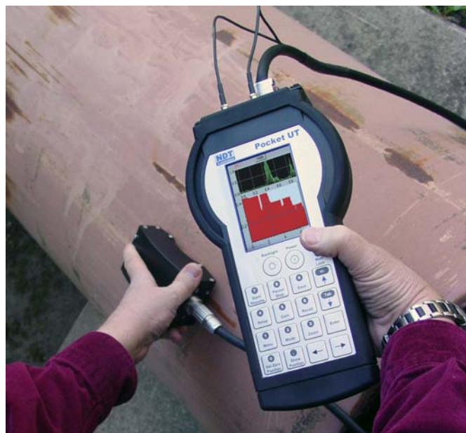
Pocket UT™ offers full C-Scan inspection capability in a portable, easy-to-use hand-held unit.
