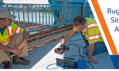
Rugged, High-Performance Single-Channel GPR Data Acquisition System
