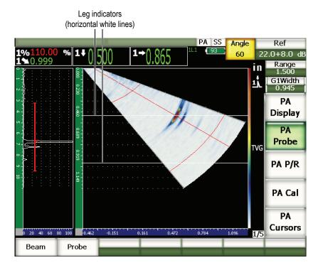
Figure 14-9 S-scan with the leg indicators active
