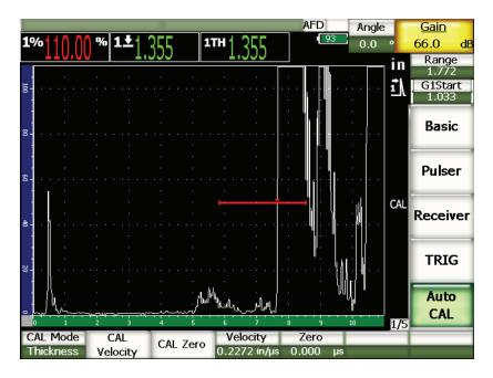
Figure 9-9 The second gated calibration signal
