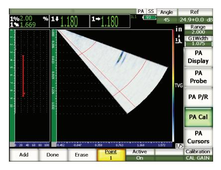
Figure 17-24 The completed gain calibration
