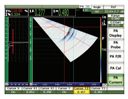
Figure 16-1 Cursors and S-scan during adjustment
