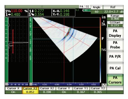
Figure 16-2 Cursors on S-scan with measurement
