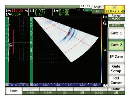
Figure 15-1 A-scan and S-scan with viewable gate
